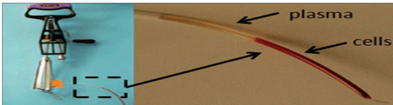
Figure 5. Plasma isolation using an egg beater centrifuge [86].
