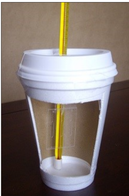
Figure 7. Styrofoam cup containing the LT microfluidic device and a thermometer
