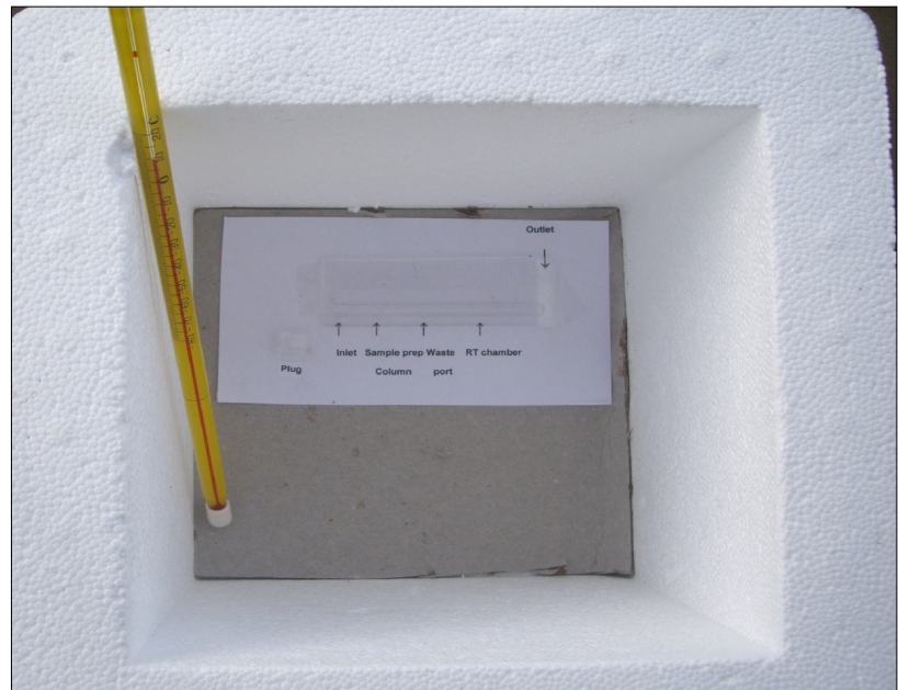
Figure 8. Styrofoam box containing the HT microfluidic device and a thermometer
